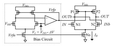
Fig. 1. FinFET SRCML inverter/buffer and its biasing circuit
