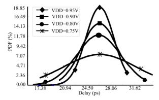
Fig. 6. PDF of stochastic delays of the FinFET SRCML AND2 gate by the corresponding standard deviation with various source voltages
