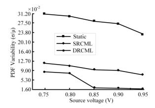
Fig. 5. PDF variability comparison of NAND2 circuit based on FinFET SRCML, DRCML, and conventional static logic
