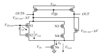
Fig. 3. Minimum operating supply voltage of FinFET SRCML circuits
