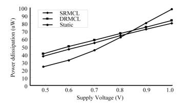
Fig. 4. Power consumption of the 1-bit full adder based on FinFET SRCML, DRCML and static logic in near-threshold and super-threshold regions
