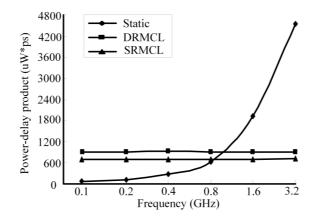
Fig. 2. Power dissipation comparisons of 1-bit full adders based on FinFET SRCML, DRCML and conventional static complementary logic in different operation frequencies
